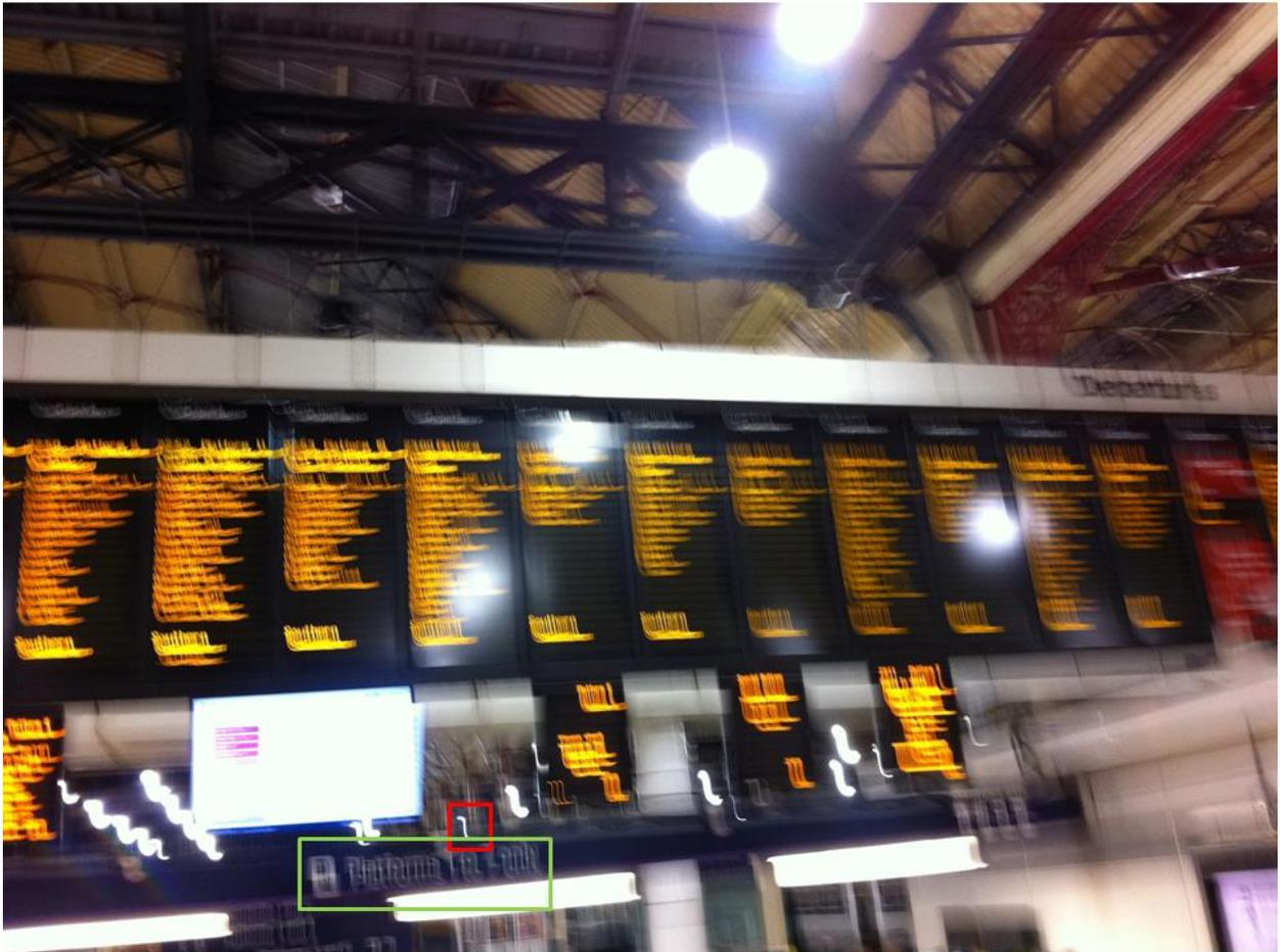
In the picture the red rectangle depicts a region which is used to estimate the motion. It is assumed that the white line in this region is representative for the motion. Therefore by thresholding this region a binary array is obtained representing the motion kernel.
